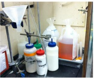
There is a higher hazard when hazardous materials are in use, as hazardous vapors are open to the atmosphere. Therefore, MAQ limits are lower for chemicals which are in use, relative to those in storage. Furthermore, closed containers located within *approved* storage are also safer than closed containers sitting out on a benchtop or on a shelf. As a result, most hazardous materials are allowed an MAQ increase when located in approved storage.
