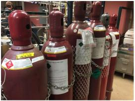
**Closed container.** A container sealed by means of a lid or other device such that liquid, vapor or dusts will not escape from it under ordinary conditions of use or handling. (Examples above for storage are closed containers.)
