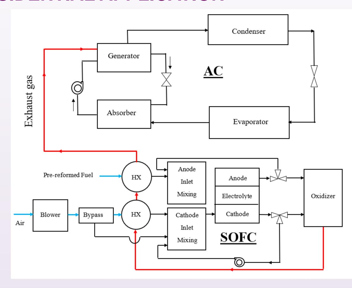
Dynamic models were developed to study dispatch characteristics and performance of integrated AC/SOFC systems. Measured dynamic power demand data from a residential apartment complex are used as an input to evaluate the dynamic operation of the integrated system.
