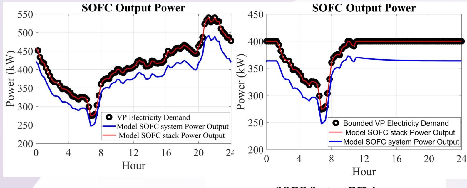
The SOFC was capable of following the highly dynamic load with an average electrical efficiency of 46%.
