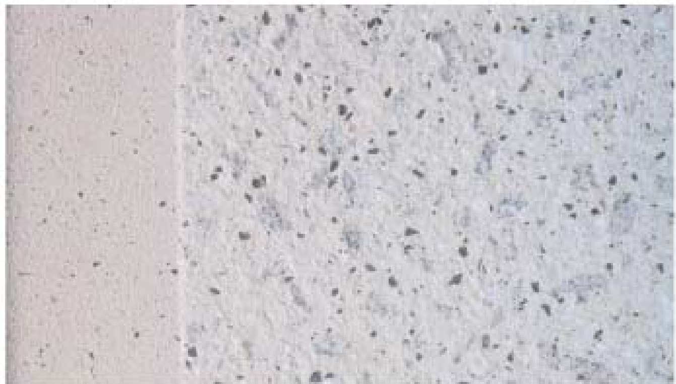
PRECAST CONCRETE ( SMOOTH FINISH )
