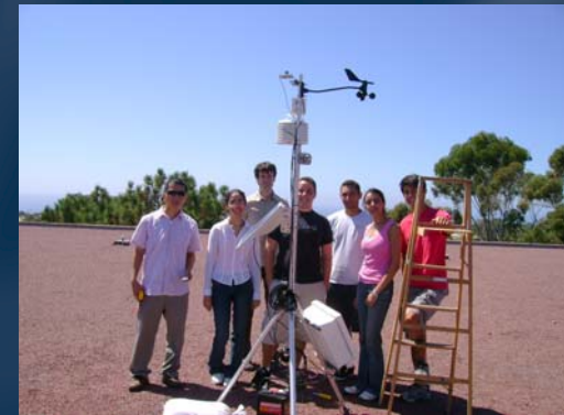
UCSD's Dr. Jan Kiessle and students at one of 30 wireless weather monitoring stations; by collecting real-time data on conditions these stations help UCSD maximize natural cooling and solar PV potential.
